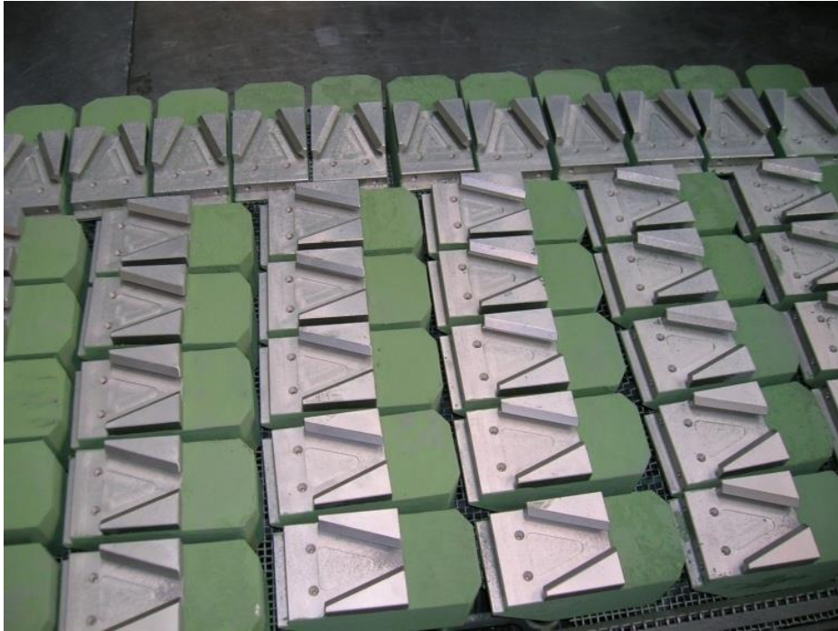
Fig. 4: Tool parts, coated with CONDURSAL N633 prior to nitriding
