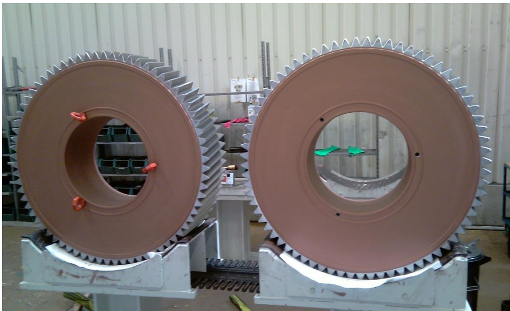
Fig. 3: Gear parts for windcraft industry, coated with CONDURSAL 0118 prior to case hardening
